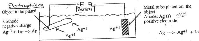
The positive ions are attracted to the negative electrode where they are reduced to a solid on the object to be plated. (The object to be plated is the cathode).
